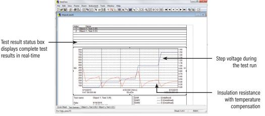
Run test and display text and graphical results from one dialog box. Model 5070 also displays step voltage.
